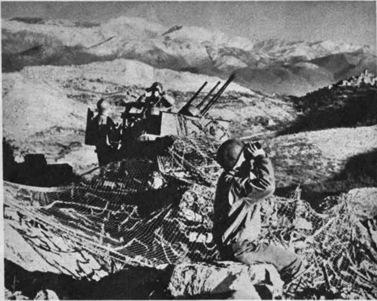
Business end of an M-15 points skyward as crew searches for German planes somewhere in Italy. With the entire chassis camouflaged, the vehicle must be recognized by its gun mount with two .50's and a 37.
